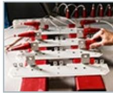
A hi-pot test is performed to make sure the finished coating has no defects, such as pin holes, voids, or thin areas near sharp corners or edges.
