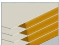
**OPEN EDGE** - Lamination extends beyond conductor farther than pinched or epoxy filled edges, and uses less tooling, which:
