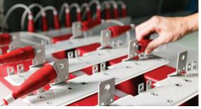
For multilayer laminated bus bars, additional tests include the partial discharge test which looks for localized dielectric breakdowns, and the insulation-resistance test which measures the layer-to-layer resistance.
