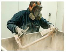
Electrically, the spray approach works well at lower voltages, up to 600-100 V with a coating which is 10-20 mil thick. Immersion in fluidized bed is a better choice for higher voltages such as 5 kilovolts (kV) and even up to 35 kV where coating thicknesses of 50-120 mils are needed.
