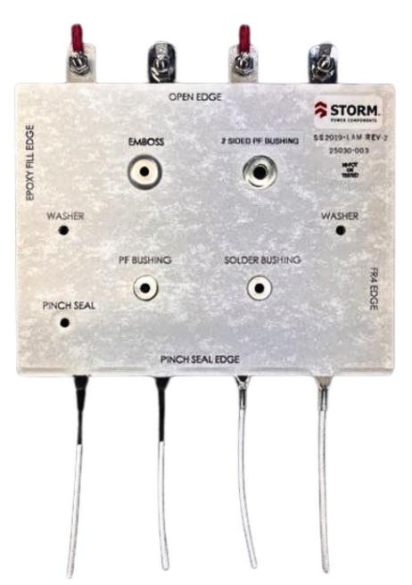
FR4 is the most mechanically robust but epoxy is more hermetically sealed and impervious to moisture
